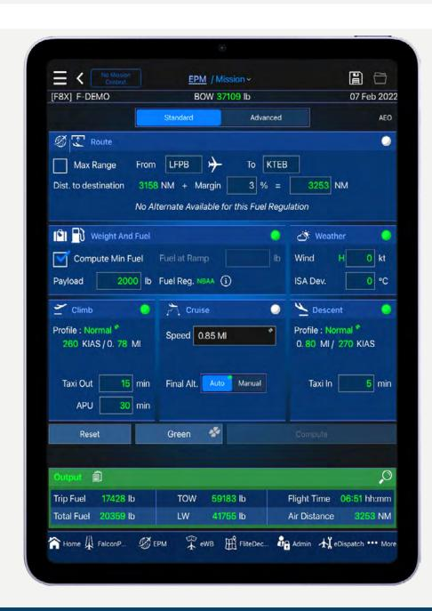
ePM is a next generation aircraft performance manual with graphical representation of high-speed performance.
