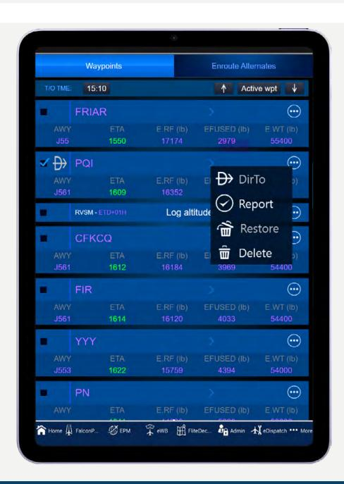
eOFP is the newest Dassault application, providing pilots with a completely digital navigation log.
